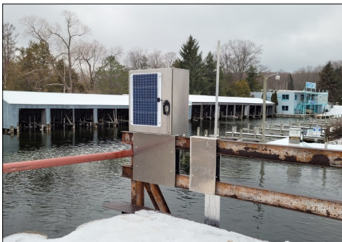
Gage at Clam River to capture water samples and conditions as part of our water quality study of Torch Lake
